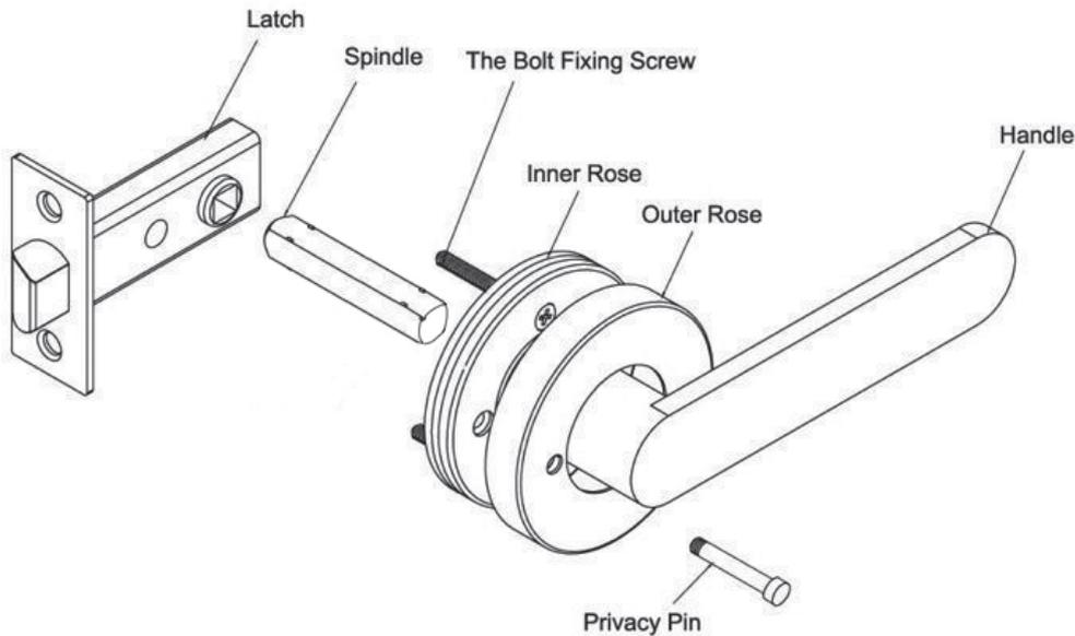
1. Using the template below, mark drilling centres into the door.
